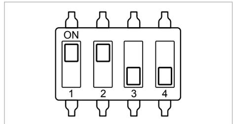
In timer mode, switch 3 or 4 must be in the 'ON' position. This mode allows for 3 different settings which will alter the time period for each segment.
